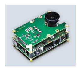
**Dimensions** 80 x 50 x 38 mm Temperature -20 to 85 °C\* **Application Range** 0.1 to 5 m\*\* Resolution 320 x 240 px 60° or 110° FoV FPS up to 60 fps ToF Chip MLX75023 Illumination 850 nm LASER
