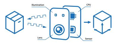
3D cameras based on Time-of-Flight technology provide depth information and intensity data for each pixel (grey value).
